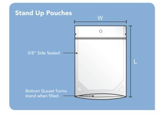
Our Stand Up Pouch offering includes the most common sizes and styles used for food packaging. All items have a K-Style configuration and hang hole, a tear notch at 1", and a zipper at 1.5". Side sealed and bottom gusseted, all our Stand Up Pouches are FDA and USDA approved.
